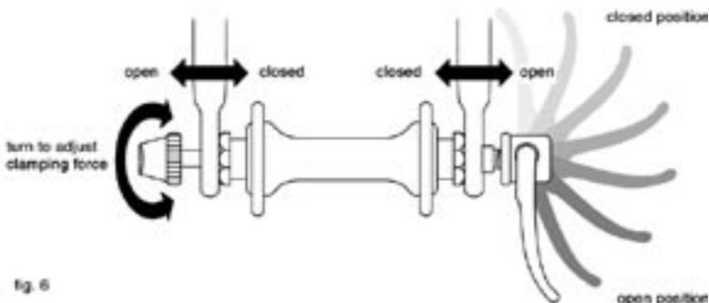
The wheel quick release uses a cam action to clamp the bike's wheel in place (see fig. 6). Because of its adjustable nature, it is critical that you understand how it works, how to use it properly, and how much force you need to apply to secure the wheel.
