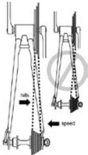
**⚠ WARNING:** Never shift a derailleur onto the largest or the smallest sprocket if the derailleur is not shifting smoothly. The derailleur may be out of adjustment and the chain could jam, causing you to lose control and fall.
