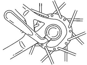
**⚠ WARNING: Securely clamping the wheel takes considerable force. If you can fully close the quick release without wrapping your fingers around the seatstay or chainstay for leverage, and the lever does not leave a clear imprint in the palm of your hand, the tension is insufficient. Open the lever; turn the tension adjusting nut clockwise a quarter turn; then try again.**
