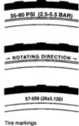
**⚠ WARNING:** Never inflate a tire beyond the maximum pressure marked on the tire's sidewall. Exceeding the recommended maximum pressure may blow the tire off the rim, which could cause damage to the bike and injury to the rider and bystanders.
